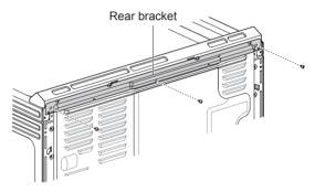
Attach the rear bracket and filler assembly as shown, using the three screws removed in step 1.
