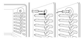
3 The meat probe icon flashes in the display if the meat probe is properly connected.
