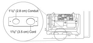
Remove the conduit connection plate
