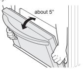
Lift door up and out until the hinge arms are clear of the slots.
