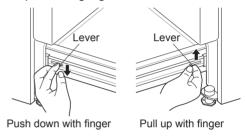
While holding both levers, carefully pull the drawer away from the range.
