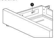
**3** Locate the glide lever on each side of the drawer. Push down on the left glide lever and pull up on the right glide lever.
