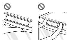
• Do not push or pull the range by grabbing the open oven door or cooktop only. Doing so can result in serious damage to the range.
